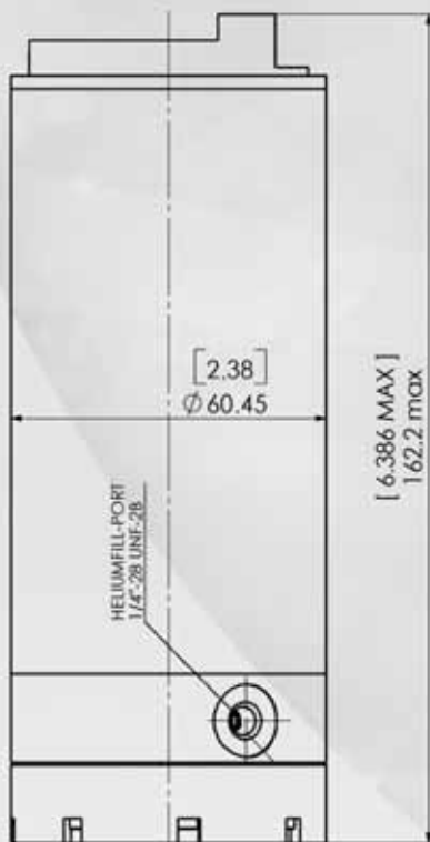
Dimensions SL150C compressor
